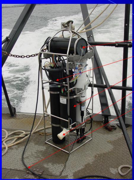
Reagent Reservoir Reagent Delivery Module ChemStar Detector Inlet Filter
